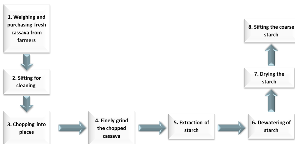
Fig. 23 - Procedure for Cassava Starch Production
